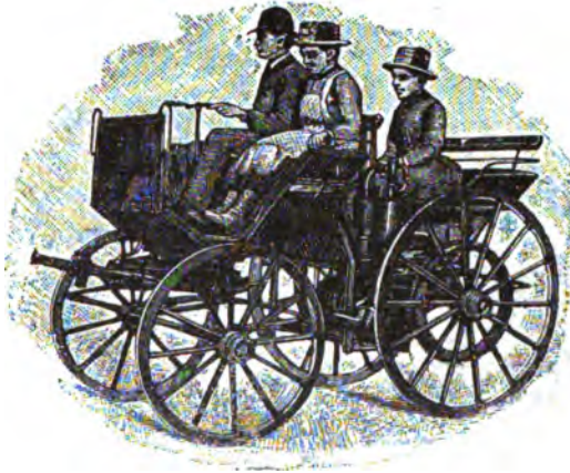
FIG. 369.—The First Daimler Motor Carriage. The motor was connected to the driving axle by two belts; one for high speed, the other for climbing; either being thrown into action as the belts were tightened by jockey pulleys, as shown in Fig. 347. Both could be thrown out of action to stop the carriage without stopping the motor. The forward axle of this carriage was centre-pivoted and turned on a fifth wheel, as in horse carriages; the steering being by upright pillar rising before the driver's seat.
